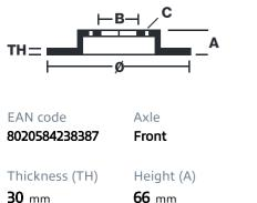
Brake disc type Centering (B) Ventilated 67 mm
