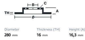
Number of holes (C) Brake disc type 10 Solid
