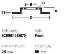
Brake disc type Centering (B) Ventilated 67 mm
